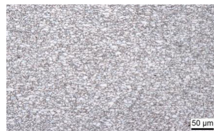
Figure 1: Microstructure images S390GD, resolution 200:1
