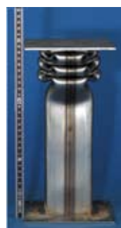
DD14 in t=2,0\text{mm} · Severe buckling · Defined formation of wrinkles (Reference made from highly ductile steel)
