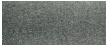
Figure 1: Passivated sample according to 504h DIN EN ISO 6270-2 AHT. White rust content < 1%.
