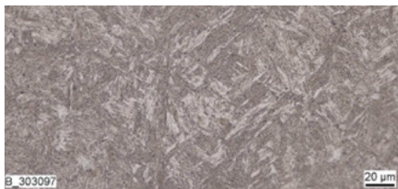
Tempered state, oil cooled 200:1
