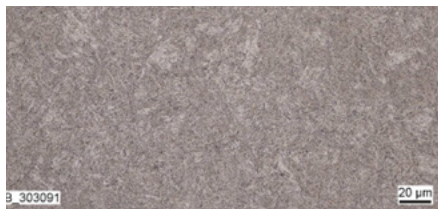
Tempered state, water cooled 200:1
