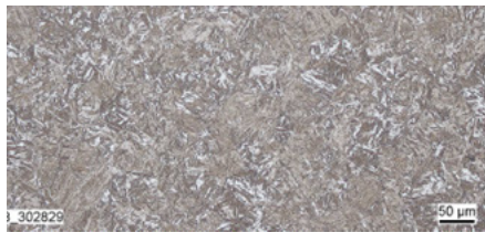
Hardened state, water cooled 200:1
