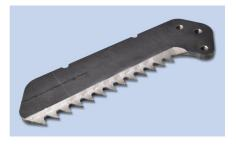
TektoSal®400 can be used as a material for counter-blades of a cutting head as shown in the picture used in a tree felling machine. The combination of wear resistance, hardness and high strength allows the machine to fell trees with a trunk thickness of several decimeter.
